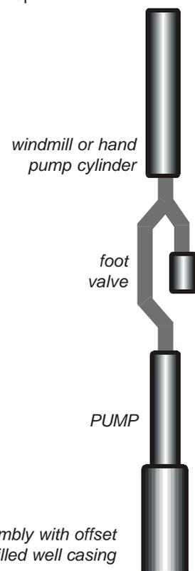
*Bypass foot valve assembly with offset elbows to fit a drilled well casing*
