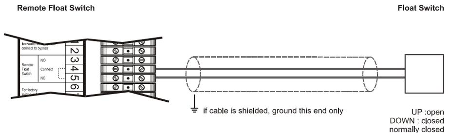
**If you are not using a float switch**, terminals 4 and 5 must be connected. Terminal 3 remains disconnected.
