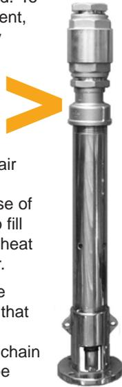
**Depth of submersion** *PS-Pumps* may be submersed as deep as necessary to ensure reliable water supply. The lift load on the pump is determined by the vertical head of water starting at the SURFACE of the water in the source. Increasing the submergence of the pump (placing it lower in the source) will NOT cause it to work harder or to pump less water. Avoid placing the pump close to the bottom where it will pick up sediment.
