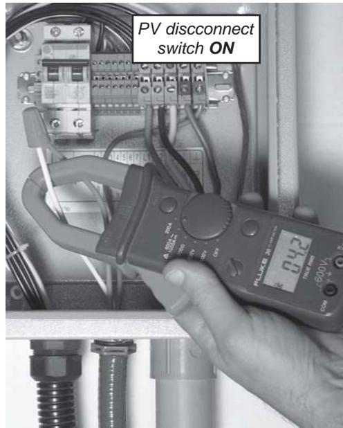
**Test 3** Same as Test 1, but disconnect switched ON
